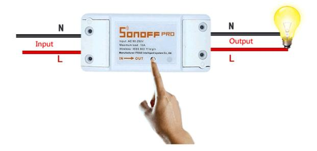
Fast press the black button on Sonoff RF for three times, the red LED is on for 3s, that means the RF controller code has been cleaned. If you failed to pair, please try to clean first.
