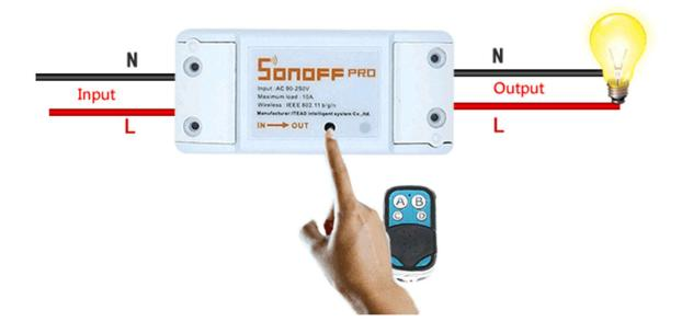
Fast press the black button on Sonoff RF twice, the red LED blinks once, then press one of the buttons of your RF controller to set pairing for 1-2 second.
