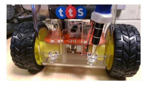
2. Carefully remove the top case of Pi2Go. This can be done by lightly pushing the case forward and when the hooks at the front are clear, pull the case up and off.
