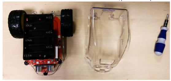
3. Unscrew the 2 screws in the battery pack and place battery pack to one side (be careful not to detach the wires attaching the battery pack to the Pi2Go)
