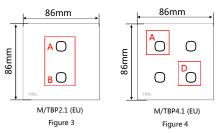
Figure 3 - 4. Dimensions - Front View (Regular version)
